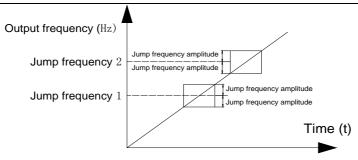
Figure 6-13 Jump frequency diagram
