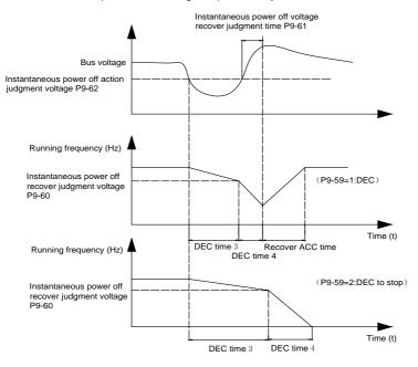
Figure 6-23 Instantaneous stop action diagrams
