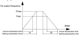
Figure 6-1 ACC/DEC time diagram
