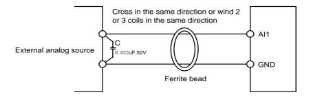
Figure 3-15 Connection of analog Input
