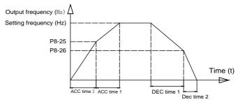
Figure 6-18 ACC/DEC time switching diagram
