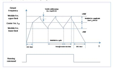
Figure 6-27 Wobble frequency operation diagram
