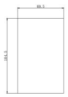
65\*100mm hole dimension of keypad bracket
