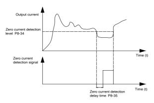
Figure 6-20 Zero-current detection diagram
