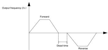
Figure 6-14 FWD/REV dead time diagram
