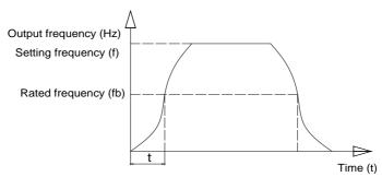
Figure 6-11 S-curve ACC/DEC A diagram
