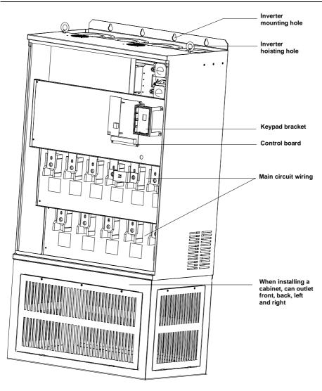
Figure 2-3 Parts of inverter
