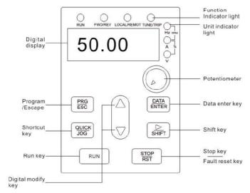
Figure 4-1 Operation Keypad Diagram
