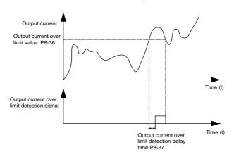
Figure 6-21 Output current over limit function diagram
