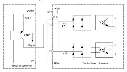
Figure 3-17 PNP type wiring
