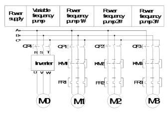
Figure 6-31 Constant pressure water supply wiring diagram
