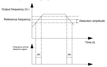
Figure 6-16 Frequency arrival detection diagram
