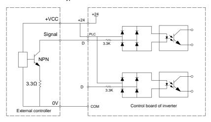
Figure 3-16 NPN type wiring
