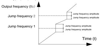
Figure 6-17 Jump frequency during ACC/DEC diagram
