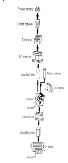
Figure 3-2 Diagram of the connection to peripheral devices
