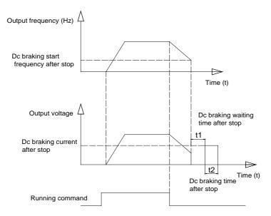
Figure 6-12 DC braking diagram
