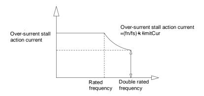
Figure 6-33 Double-speed over-current stall action diagram
