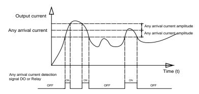
Figure 6-22 Any arrival current detection diagram
