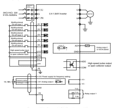
Figure 3-3 Wiring Diagram (1AC/3AC 220V 0.4~1.5kW)
