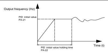
Figure 6-26 PID initial value function diagram
