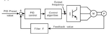
Figure 6-24 PID control diagram
