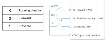
Figure 6-8 Three-line Running Mode 2
