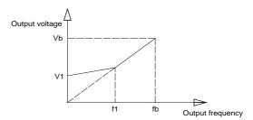
V1:Manual torque boost voltage
