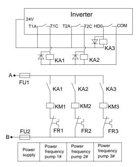
Figure 6-32 Constant pressure water supply electrical schematic diagram
