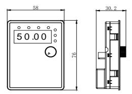
Keypad dimension of 1AC/3AC 220V 0.4~1.5kW inverters
