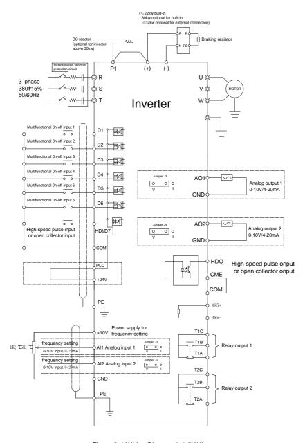
Figure 3-4 Wiring Diagram (>1.5kW)
