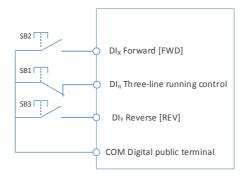
Figure 6-7 Three-line Running Mode 1
