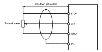
Figure 3-14 Connection of analog input
