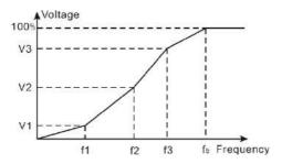
Figure 6-4 V/F curve setting diagram
