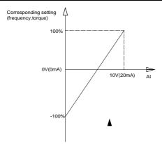
Figure 6-9 Corresponding Relationship between Analog Reference and Setting
